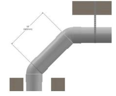
Install Cleanout ports every 50 feet on angled runs. Straight trunk lines can run up to 100 feet with cleanouts at either end.
